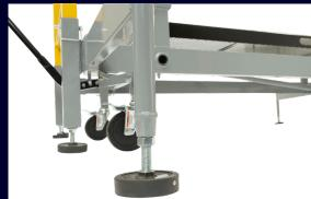
Releasing the handle raises the casters, locking the base in place automatically without the need to manually lock / unlock casters.
